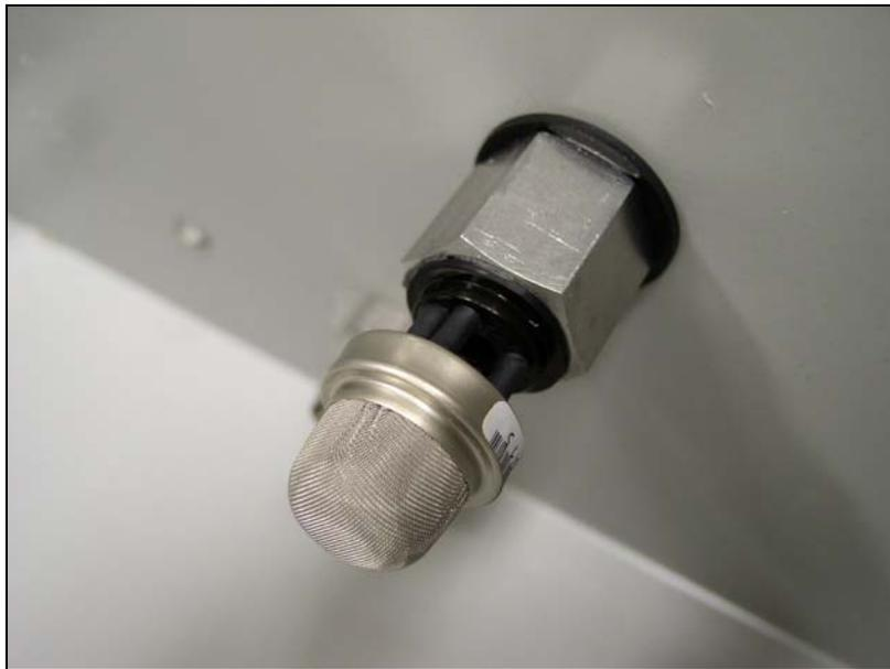
Figure 15: Remote Sensor Mount
