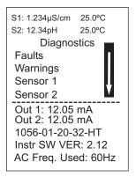
Information about each condition is quickly accessible by pressing DIAG on the keypad. User help screens are displayed for most fault and warning conditions to assist in troubleshooting.
