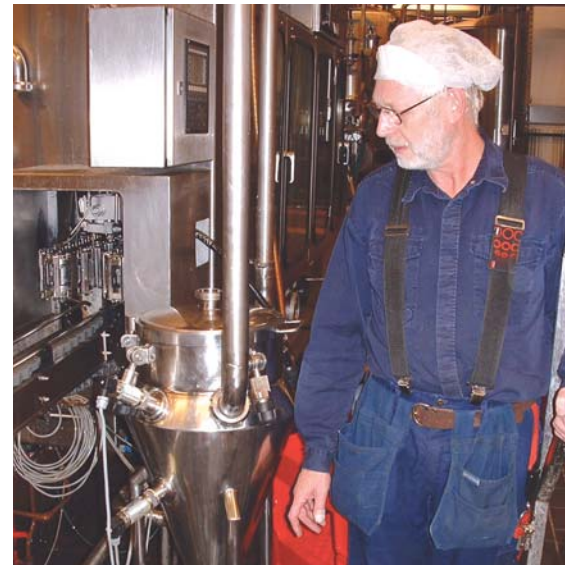
Figure 2: The hygienic vibrating fork level switches mounted in the overspill tank.
