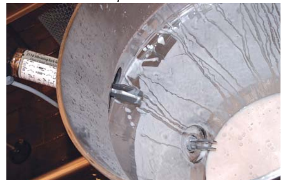
Figure 3: The inside of the tank showing the hygienic vibrating fork.
