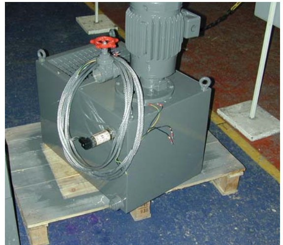
Figure 2: The Compact Vibrating Fork Level Switch used in a smaller filtration unit.
