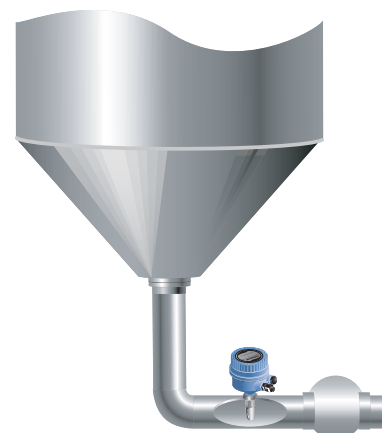
Figure 2: Rosemount 2120 mounting for successful low-level drain.
