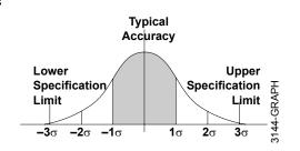
Note: Accuracy distribution shown is for 244E, Pt 100 RTD sensor, range 0 to 100  $^{\circ}$ C.
