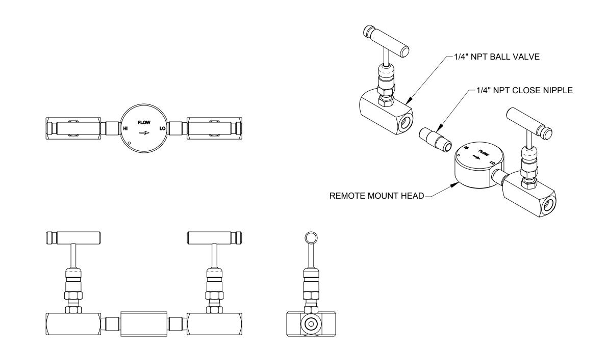
REMOTE MOUNT ELECTRONICS CONNECTION PLATFORM WITH NEEDLE VALVES
