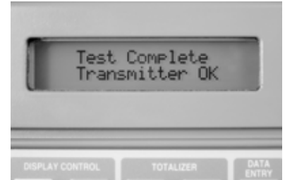
Transmitter Calibration is verified.
