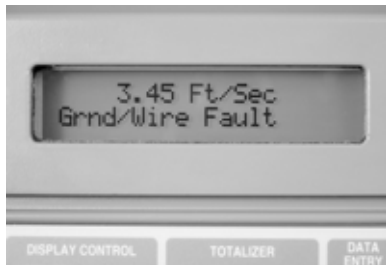
Grounding and wiring fault displays on LOI.
