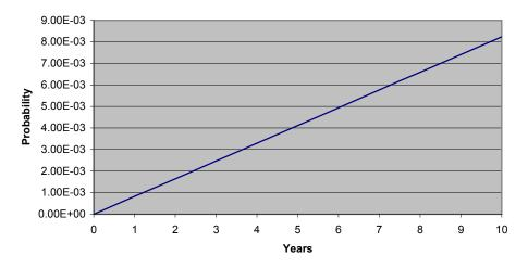
Figure 1: PFD<sub>AVG</sub>(t) 8712D Magnetic Flow Transmitter – DC power option
