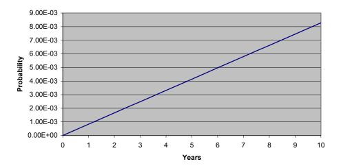
Figure 2: PFD<sub>AVG</sub>(t) 8712D Magnetic Flow Transmitter – AC power option
