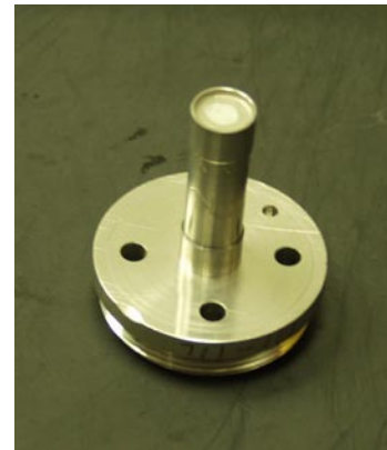
Acid-Resistant Stoichiometer Cell
