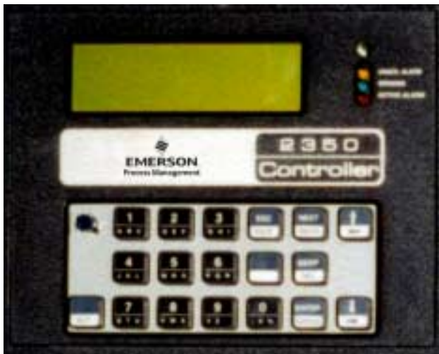
The Model 1000 gas chromatograph can either have the 2350A controller built into the face of the analyzer (shown) or mounted remotely in a 19" rack enclosure.
