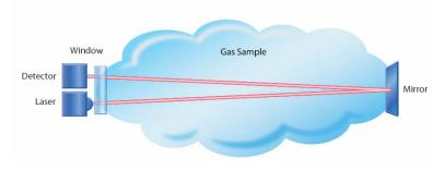
water vapor in a sample of air can be measured. As shown above, a beam light is passed through a sample and the amount of light lost (absorbed by the target gas) is measured by a detector. The target gas does not absorb all light, but a predictable amount of very specific wavelengths of light. If the light's wavelength is adjusted, the amount of light (power) observed on the output will vary accordingly.
