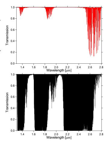
traditional techniques do not work because methane has a much stronger absorbance in the same regions on the graph and completely drowns out the measurement.
